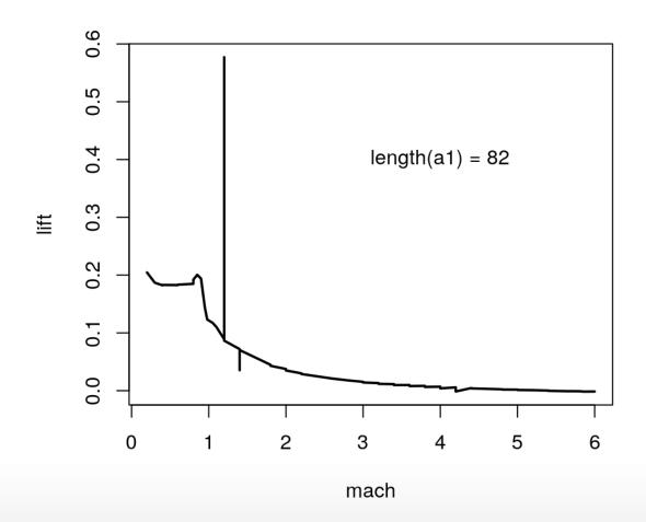
Cart3D.v2 was more stable; and run on an fully automated adaptive grid of just 780 points.
