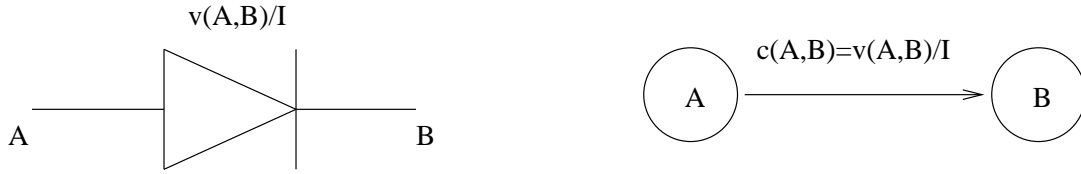
Figure 3: (Left) Electrical representation/notation for a diode with terminals A and B . v(A, B) \equiv v_{AB} , (the voltage drop from terminal A to terminal B ). (Right) Graphical (edge/arc) representation/notation of the diode on the left.
